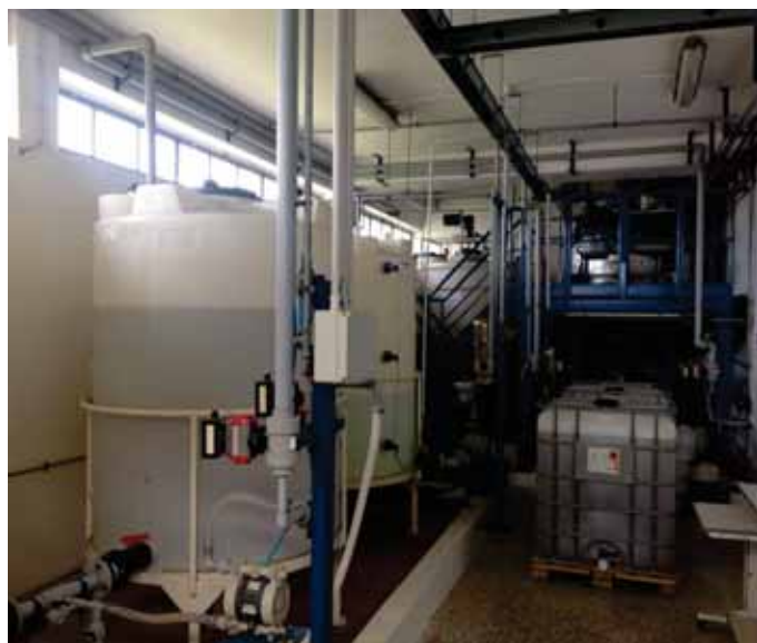
Figure 4. Industrial pilot plant to produce chitin nanofibrils.
